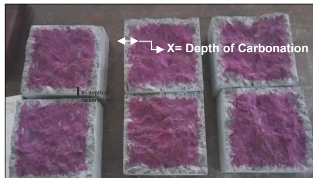
Figure 1. Phenolphthalein Sprayed Cube Sample
