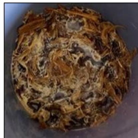
Figure 2. Soaking of Kenaf Fibre in 1.0M NaOH Solution
